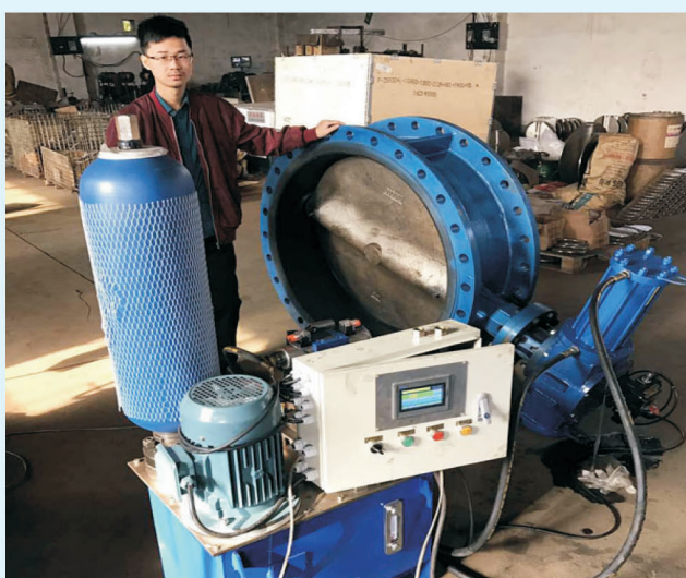
蓄能式液控蝶阀带PLC控制箱 Accumulation Type Hydraulic Butterfly Valve with PLC Control Box
