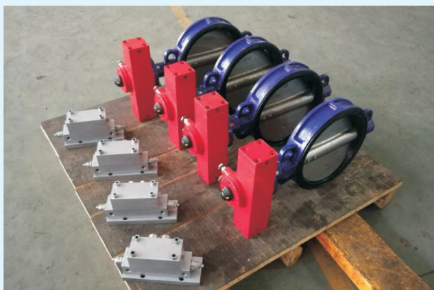
液动蝶阀带控制块 Hydraulic Butterfly Valve with Control Block
