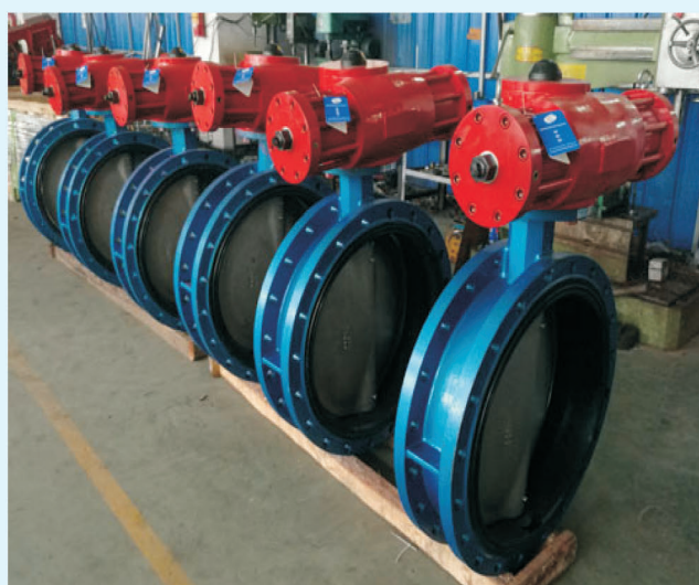
出口型船用液动蝶阀 Hydraulic Butterfly Valves Special for Shipyard
